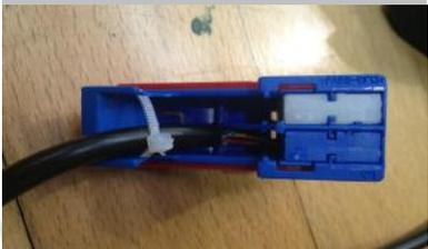
Using a small sharp object, bend the retaining tag (seen below in blue at the tip of the blade) away from the white plug slightly and then slide out the white block connector. This can be discarded.
