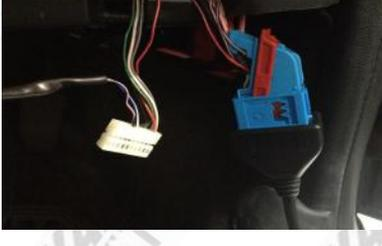
and then slide the vehicles WHITE plug (seen above on the left) into the ADC195 male connector.
