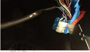
Once the white connector is out of the vehicle plug, connect the vehicles BLUE plug to the ADC195 female cable (seen below on the right):
