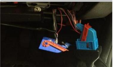
Lastly, fit the blue male connector of the ADC195 (seen above on the left) into the vehicle BCM and then connect the OBD lead. You can then continue to read the PIN from the BCM by selecting option 2 (Y-cable)
