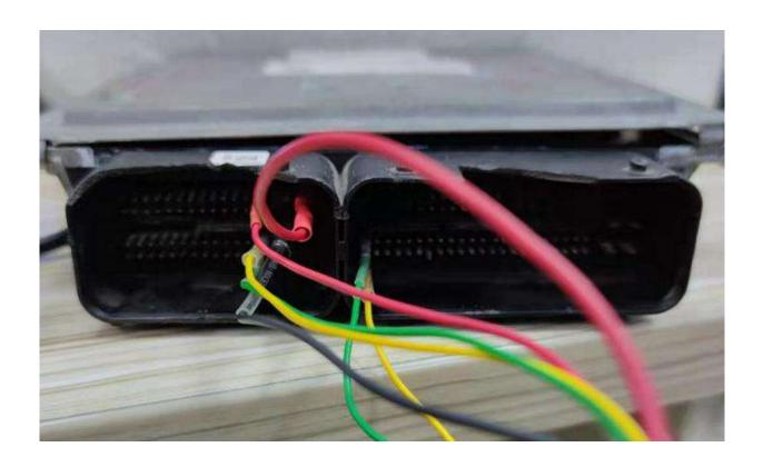
1.4 In second diagram, Need to remove ecu cover and add a 2.2K resistor, a 100NF capacitor and a TJA1050 communication chip, and short circuit in place that marked in diagram. The complete operation can only be carried out after the wiring here is completed (Need to plug 12V to AT200).
