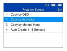
Select Copy by Activation from programming list. Activate or Trigger sensor to be copied.
