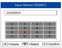
Press **Trigger** to select the numbers, press **N** to exit and once a number is selected, the **N** button can be used to delete the entered number. After all the numbers are entered, press **Y** to confirm.
