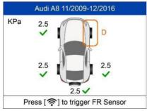
All sensors have been triggered. Display advances to connect OBD cable for diagnosis even if not all sensors have been successful activated.
