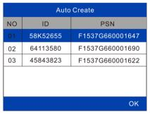
Once the sensors are successfully programmed, the sensor IDs and the PSNs (Product Serial Number) will display on the tool.
