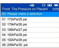
Use the **UP/DOWN** button to select the correct tire pressure on placard and press **Y** to confirm and turn to the previous menu.
