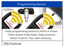
Place a new CGSULIT sensor near the top of the tool to program.
