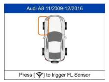
Press **Trigger** to activate the sensor.
