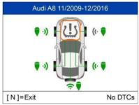
If no DTC(s) is present in the ECU, the middle TPMS icon displays gray and a "No DTCs" message displays at the right bottom of the screen.
