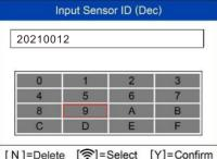
Press **Trigger** to select the numbers, press **N** to exit and once a number is selected, the **N** button can be used to delete the entered number. After all the numbers are entered, press **Y** to confirm.
