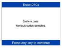
The tool will automatically re-check the ECU to ensure all DTCs have been deleted.
