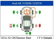
Green signal and OBDII icons: the ECU ID matches Sensor ID.
