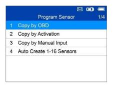
There are four ways to program CGSULIT sensors: Copy by OBD, Copy by Activation, Copy by Manual Input and Auto Create 1-16 Sensors.
