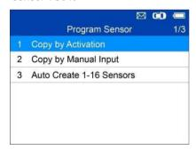
Press Y to select Copy by Activation. Place the tool near the sensor to be copied. If the sensor is still attached to the wheel, hold the tool close to the tire sidewall right above the sensor.
