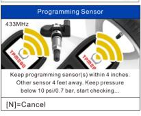
Place a new CGSULIT Sensor TS01 in the sensor slot or hold the top of the tool close to the sensor to program.
