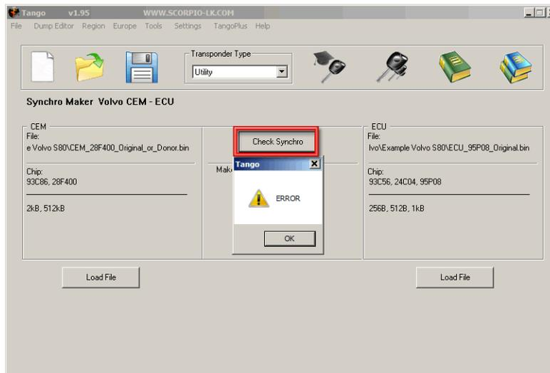
To actually synchronize the files press the arrows beneath "Make Synchro". The upper arrow that points left will prompt saving a **new CEM dump** file that is synchronized with the ECU. The second button which points right may be used to create a new ECU dump file instead. Choosing which function to use (create new CEM file or
