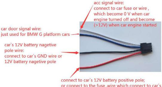
or connect to the fuse ,wire which connect to car's 12V battery positive pole. this wire must keep power on.
