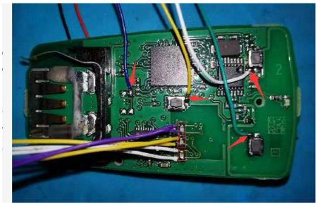
If your circuit board is the same as next picture ,you can connect the 3D A B C wires as this picture
